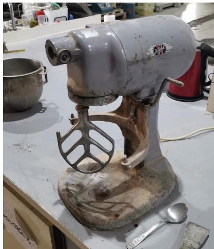
Figure 3.20. Tabletop mixer that is used to mix mortar samples.
