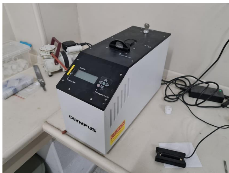
Figure 3.15. Olympus BTX III Benchtop XRD Analyzer used for the XRD analyses.
