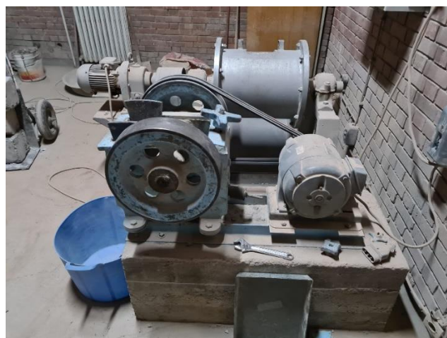
Figure 3.8. Mechanical crusher used for the crushing procedures.
