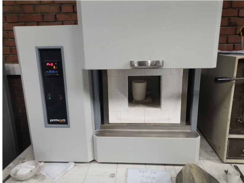
Figure 3.12. Protherm MoS Series Chamber Furnace used for the clay calcinations.
