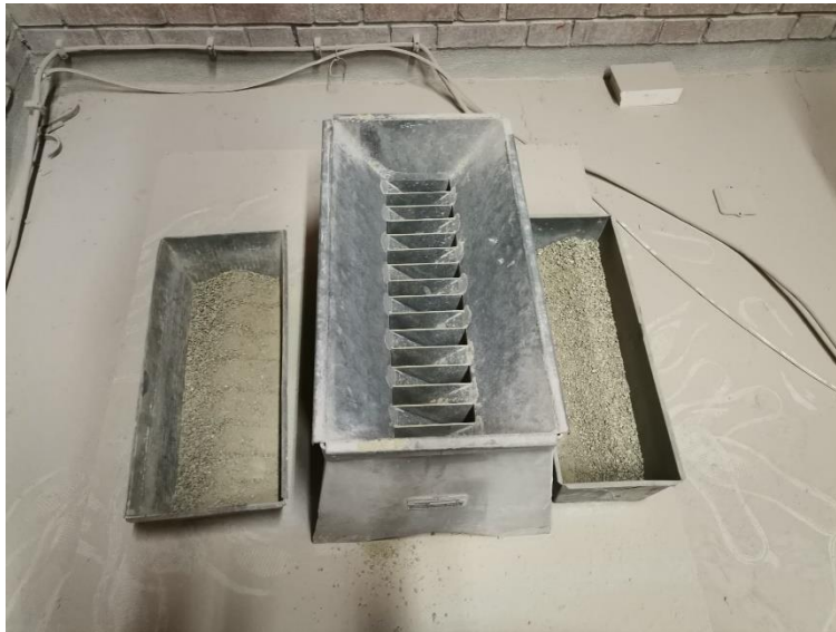
Figure 3.9. Mechanical splitter used for the quartering procedures.
