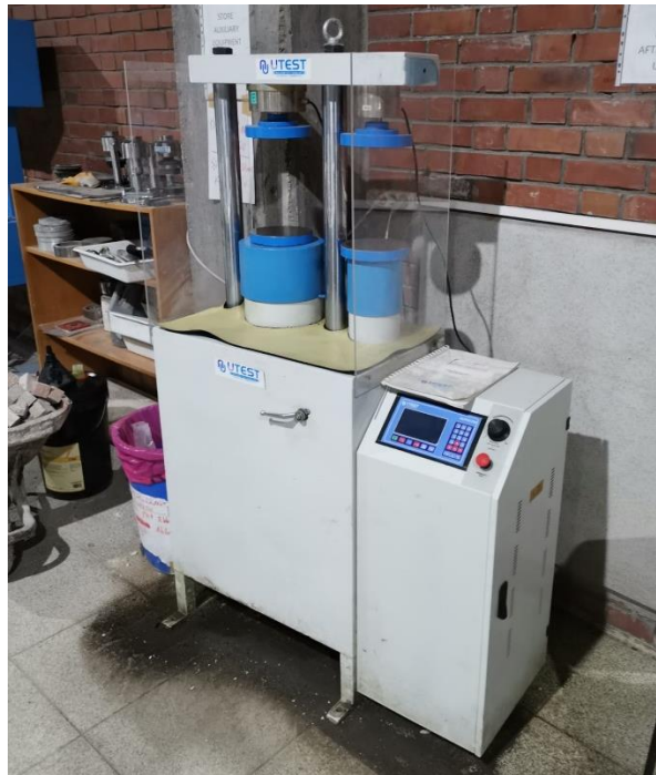
Figure 3.23. UTEST UTCM-3742.FPR Automatic Cement Flexure/Compression Testing Machine.
