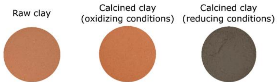
Figure 3.13. Color change of raw clay with the calcination under a) oxidizing b) reducing conditions (Hanein et al., 2022).
