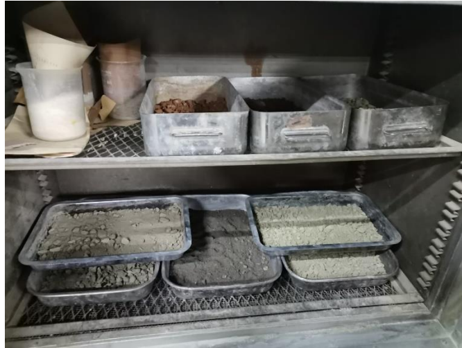
Figure 3.10. Clay samples are dried in the 120 °C oven before the grinding.
