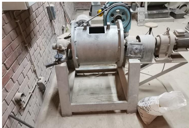
Figure 3.11. Rotary ball mill grinder equipment that is used in the study.
