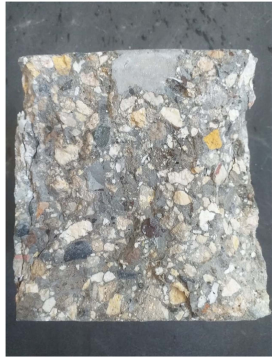
Fig. 12. Fracture surface of 100% RCA sample after compressive strength testing.
