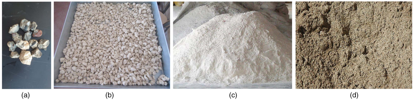
Fig. 1. Fine and coarse aggregates used in this study: (a) RCA; (b) NA; (c) natural calcareous sand; and (d) river sand.
