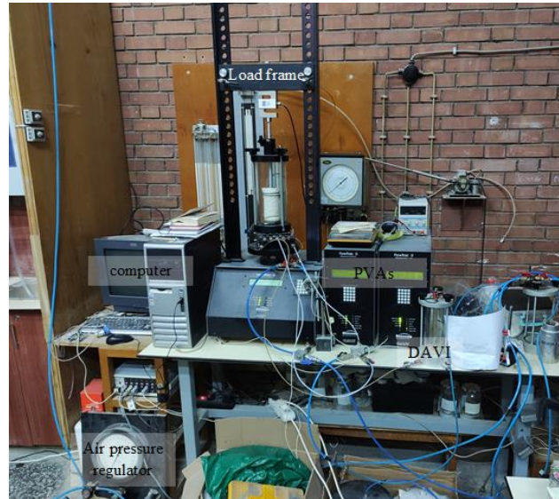
Figure 3.38 The picture of the unsaturated triaxial test setup
