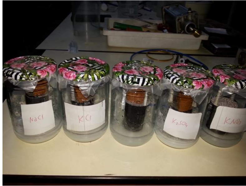
Figure 3.24 Implementation of vapor equilibrium technique for Ankara clay specimens
