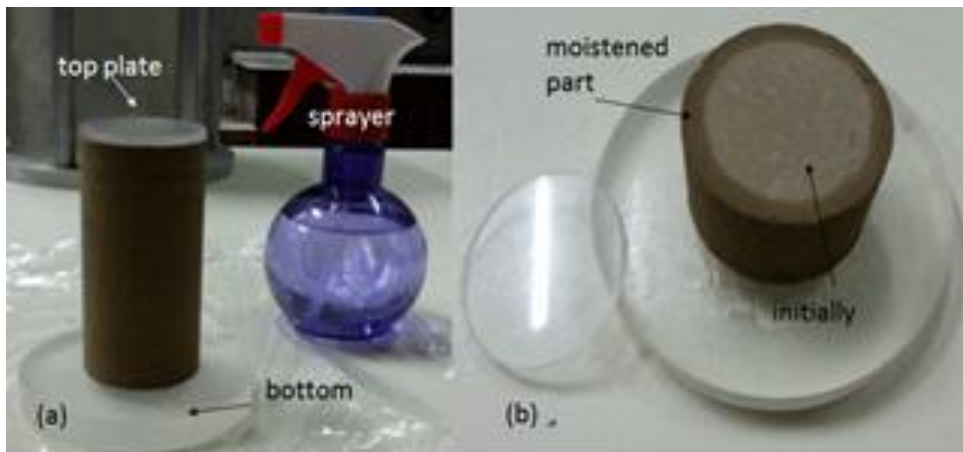
Figure 4.3 Equipment (a), the top view of specimen immediately after spraying (b) Mersin silt was used and dry densities of specimens prepared by compaction were in the range of 1.50 to 1.58 g/cm 3 . The water content was increased from an initial value of 5% during compaction to about 13% at the end of water content equilibration (Fig. 4.4). The maximum error for the water content became 0.9% (Fig. 4.4-a) and 0.8% (Fig. 4.4-b) after 1 day and 2 days water content equilibration, respectively.
