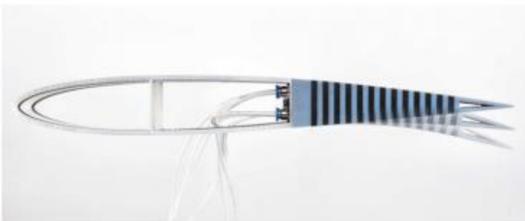
Figure 1.10. Deformation of 3D Printed Trailing Edge Specimen [18]
