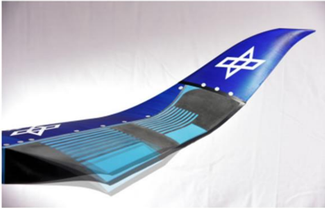
Figure 1.11. 3D Winglet Specimen Built Using Pressurized Cell Structures [18]
