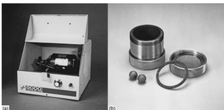
Figure 1.10. SPEX 8000 mixer mill. (b) Tungsten carbide vial set consisting of the lid, vial, balls, and gasket. Courtesy of SPEX CertiPrep, Metuchen, NJ.
