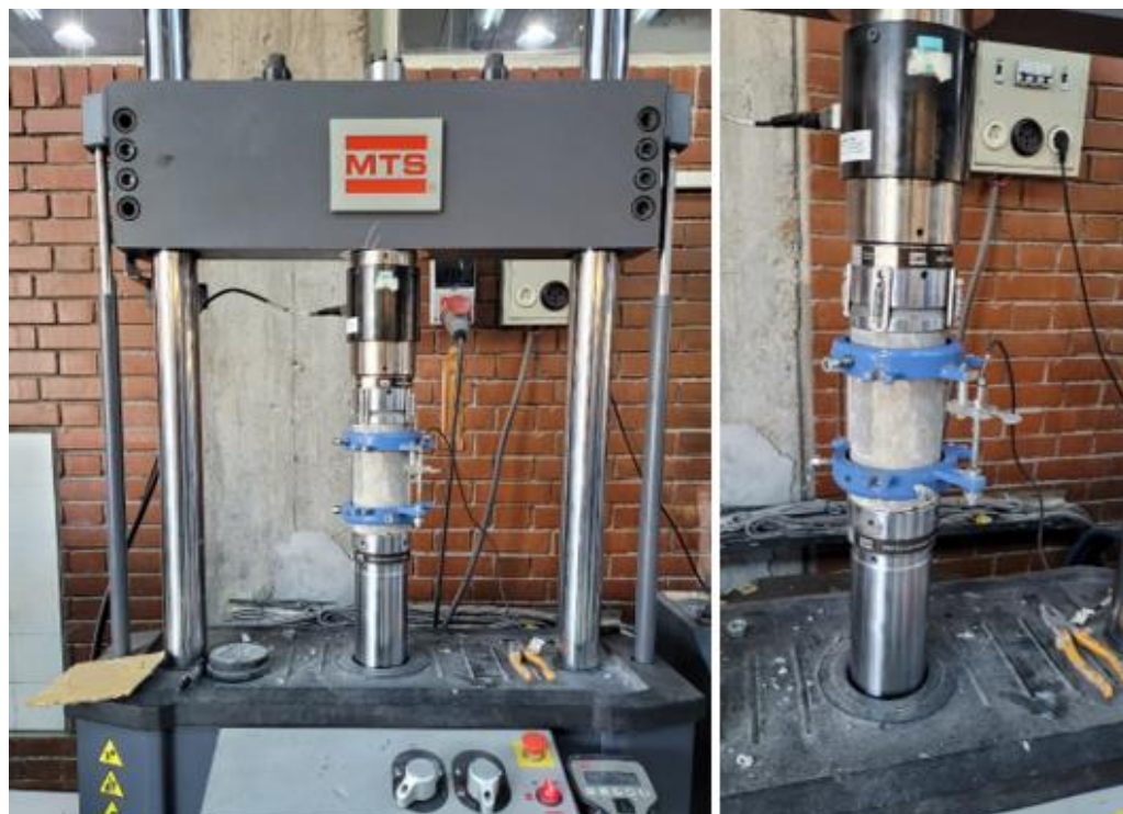
Figure 3.15 Static Modulus of Elasticity Experimental Setup
