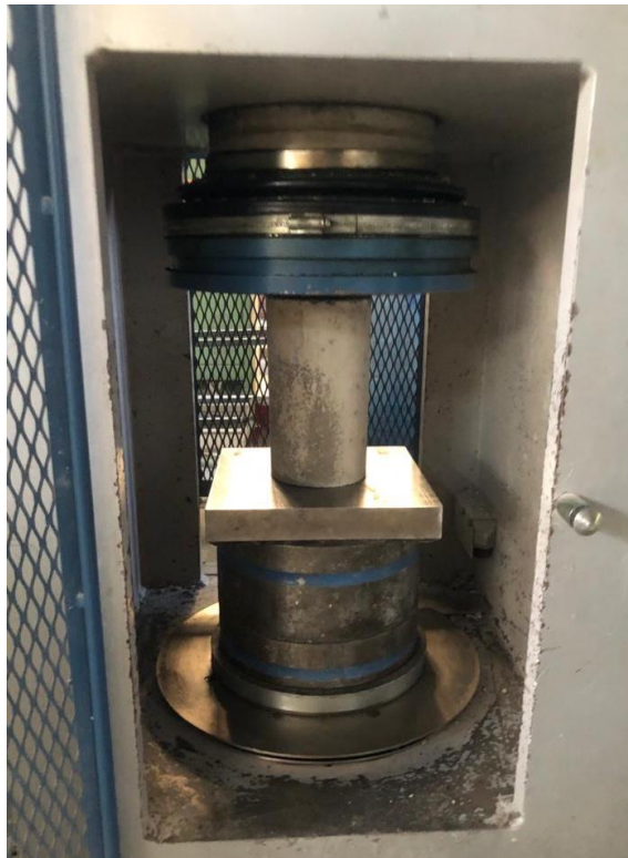
Figure 4.10 Testing Specimen in the UTS Machine
