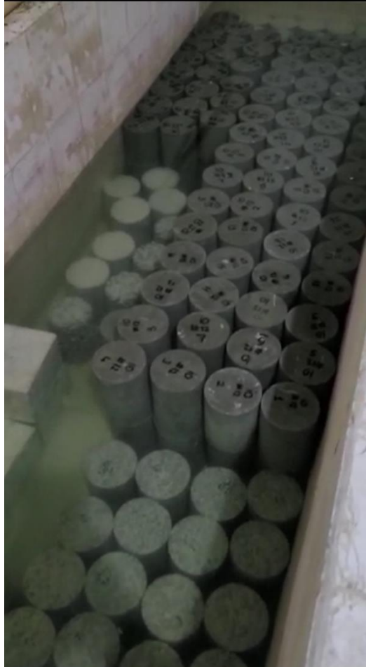
Figure 4.7 Curing Specimens in the Water Storage Tank
