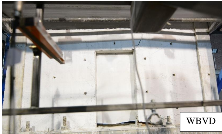
Figure 3.6. Failure State of Clay Brick Infill Walls (continued)
