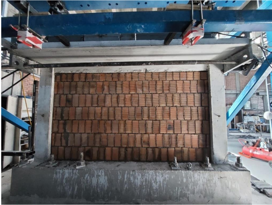
Figure 2.15. Built WBVN2 Without Plaster on it
