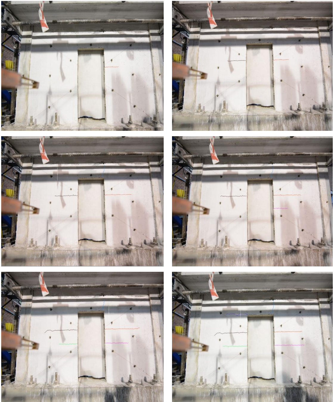
Figure 2.37. Crack Path of WPVD
