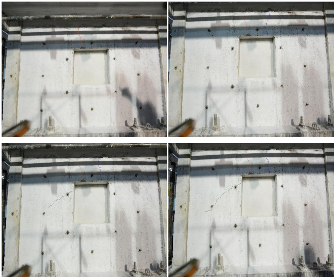
Figure 2.21. Crack Path of WBVW Experiment
