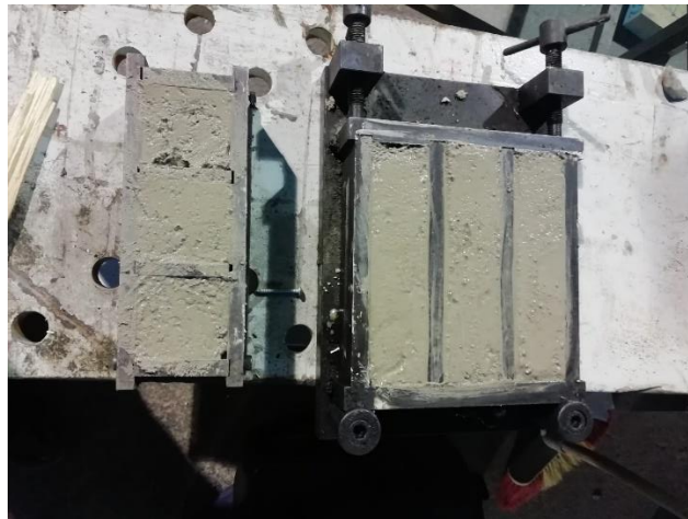
Figure 2.7. Cube and Prismatic Specimens of Constituents
