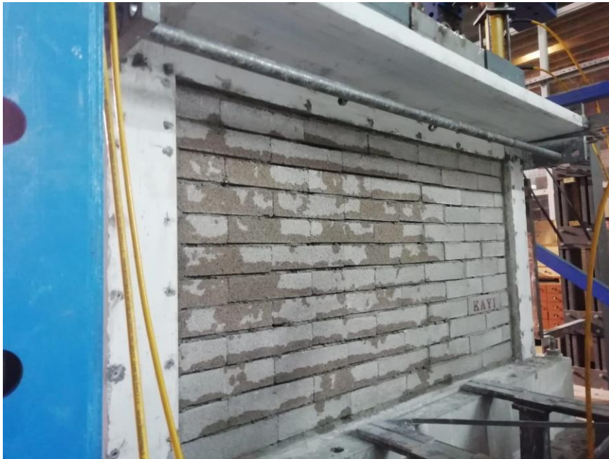
Figure 2.27. Built WPVN Without Plaster on it
