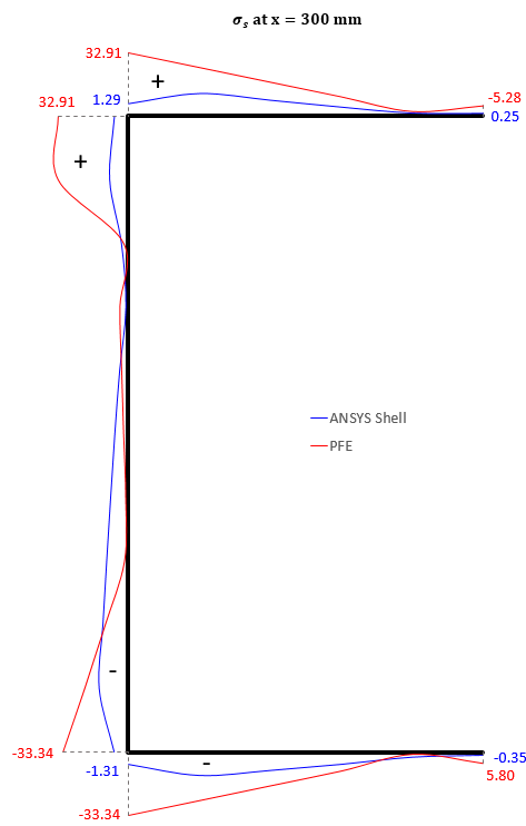
Figure 4.33. Comparison of \sigma_y normal stresses for Example-8
