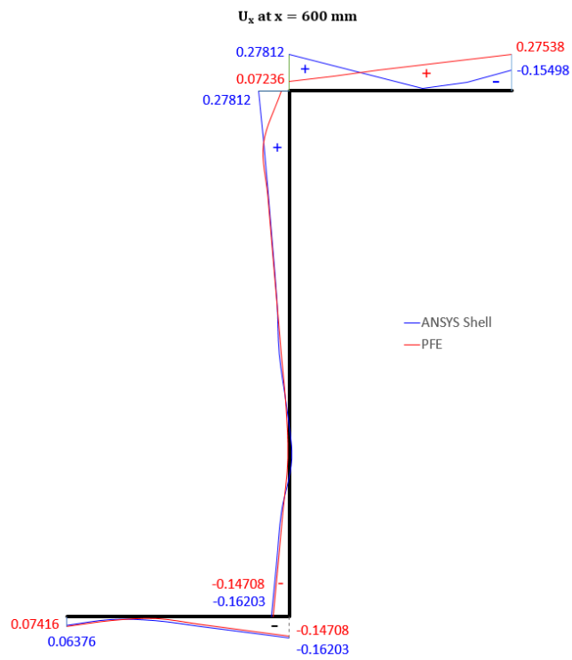
Figure 4.38. Comparison of U x displacements for Example-9
