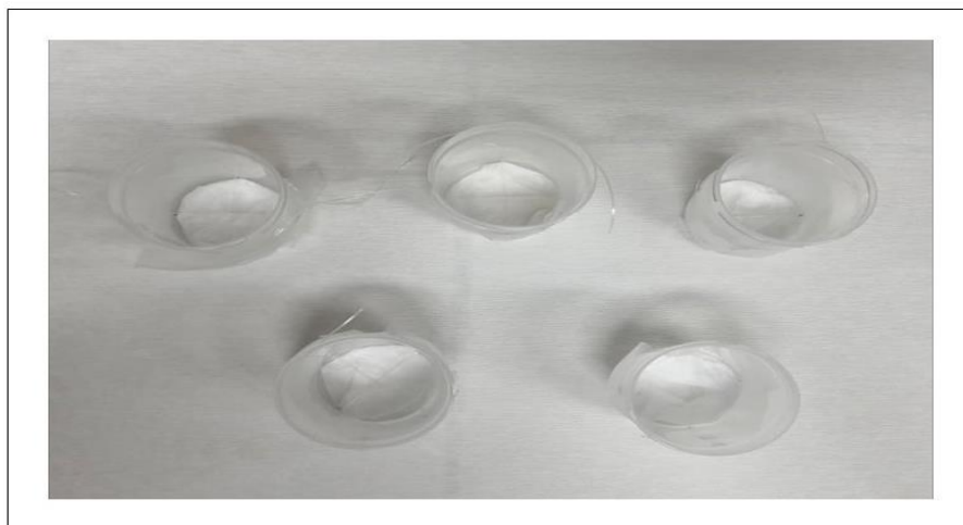
Figure 2.4. Five scaffolds placed in each container, before addition of the gelatin solution.
