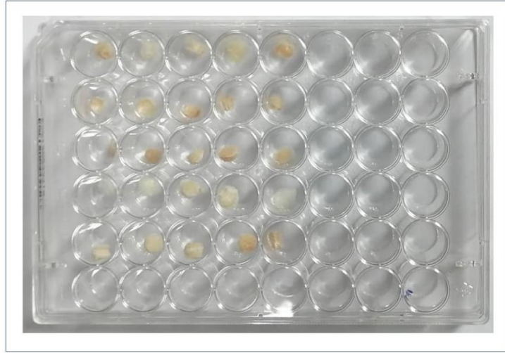
Figure 2.6. Final gelatin coated scaffolds, after 14-16 h of freeze drying
