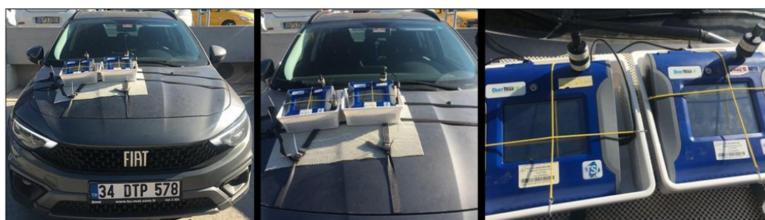
Figure 17. Created kit on the car's hood to take mobile measurements
