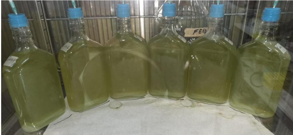
Figure 3.6. Set 3 after the setup. From left to right: R7.00-1, R7.00-2, R7.70-1, R7.70-2, R8.50-1 and R8.50-2. Reactors were arranged in a crescent pattern to distribute light equally.
