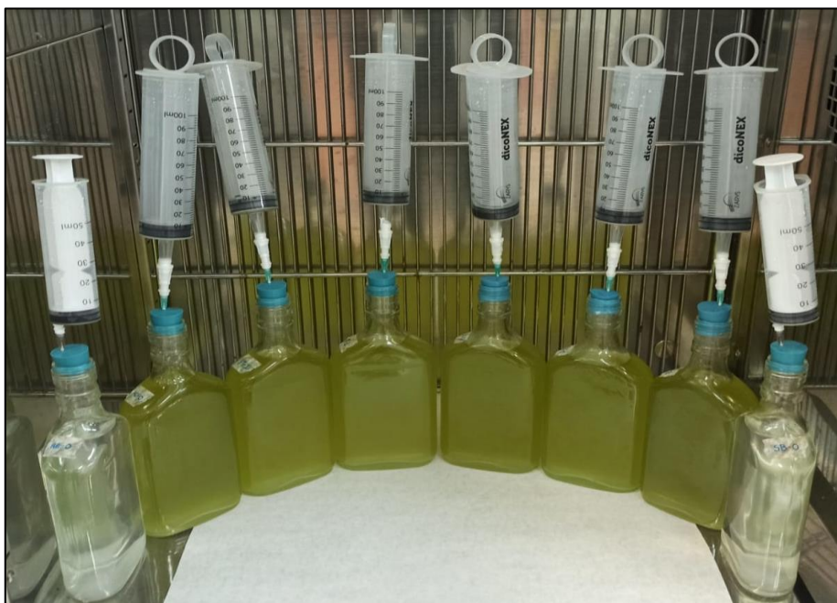
Figure 3.5. Set 2 after the setup. From left to right: Acetate-containing C0, T0, T1, T2 and sucrose-containing T0, T1, T2 and C0. Reactors were arranged in a crescent pattern to distribute light equally.
