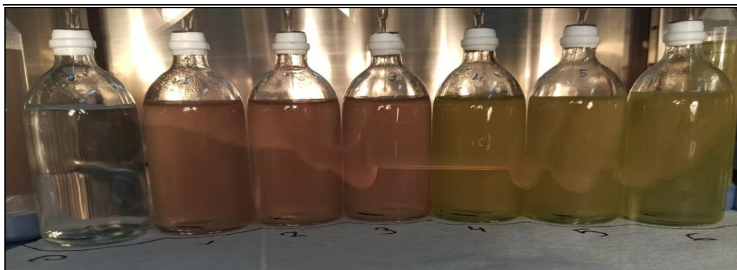
Figure 3.4. Set 1 after the setup. From left to right: control reactor, triplicate WT strain reactors, triplicate YO3 strain reactors.
