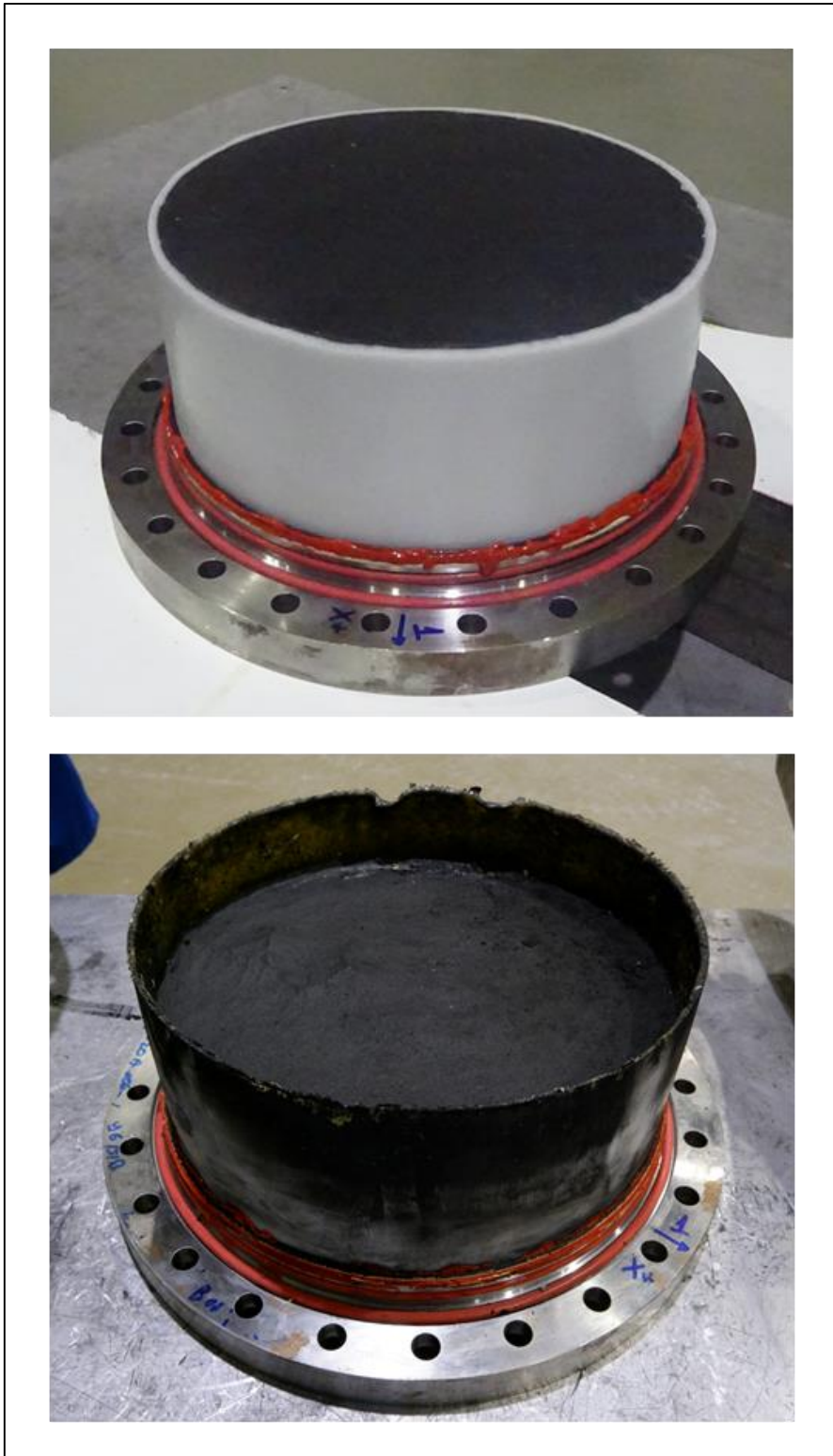
Figure 3.5. The propellant grain before and after the static firing
