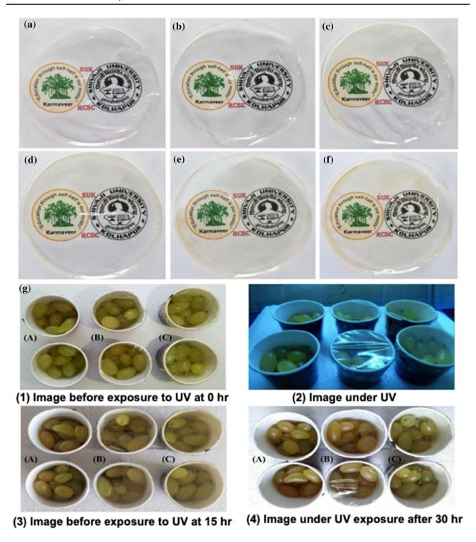
**Fig. 7** Photographic images demonstrating the transparency of PVA films without any additive: a PVA@WTR-CDs composite films, **b-f** as the concentration of WTR-CDs rises (0.5, 1.0, 2.0, 3.0, 5.0 mg), and **g** Digital images showing the efficacy of produced composite green synthesized CD-based films in food packaging applications
