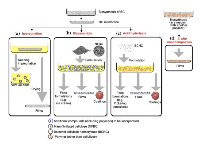
Fig. 4 Techniques for mixing bacterial cellulose with other components for use in food packaging, A Impregnation; B Disassembly; C Acid hydrolysis and D In situ nanocomposites. Adapted from [130], reproduced with the permission from Elsevier
