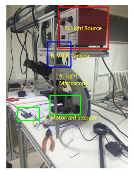
**Figure 1.** Data Acquisition system. A, Light microscope; B, VNIR Camera; C, Motorized Stepper; D, Light Source.
