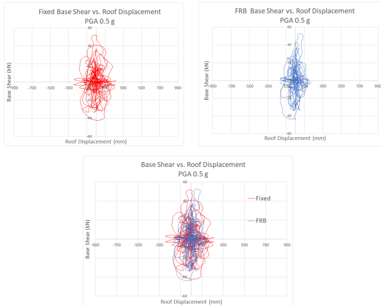
Figure 6.17: FRB and Fixed base shear force versus roof displacements for the 8 story 1 bay case
