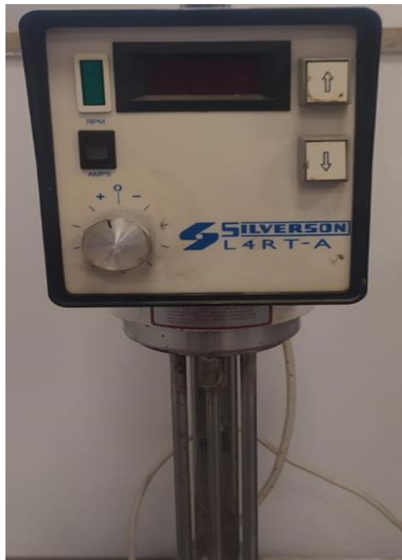
Figure-4: Silverson high shear mixer
