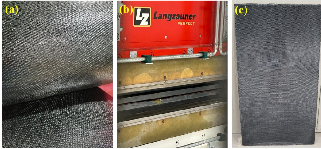
Figure 2.2 Production of PPS/CF laminates; (a) Prepreg lay-up, (b) Consolidation by compression molding, and (c) A laminate produced.
