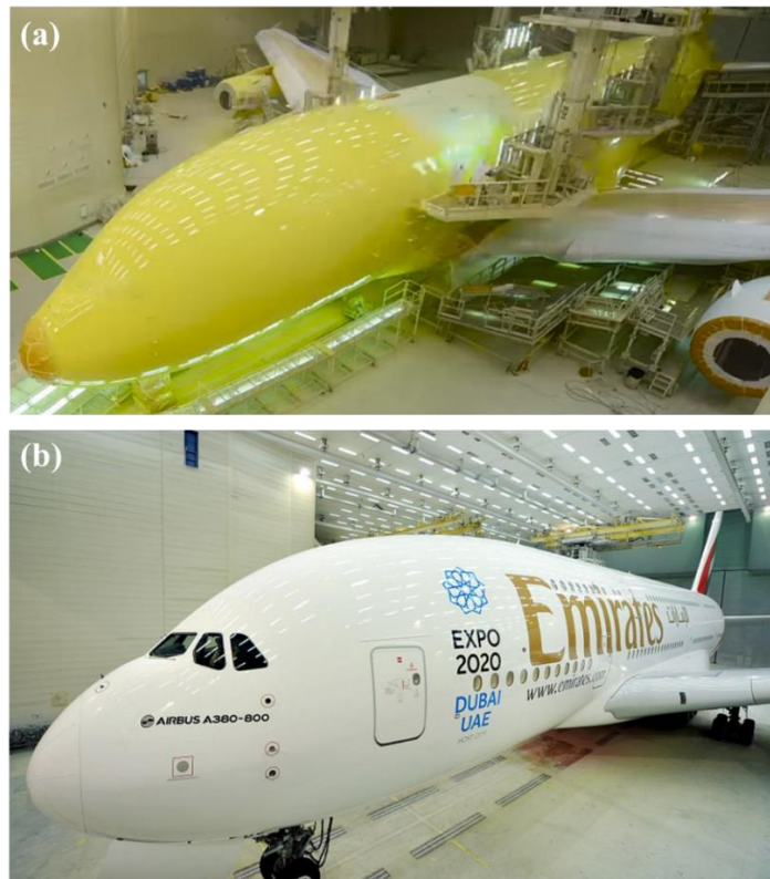
Figure 1.2 Images of an aircraft, after (a) primer painting and (b) top-coat painting.
