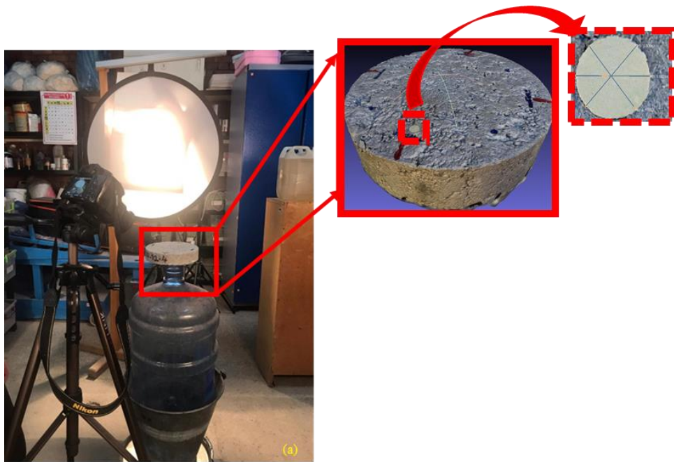
Figure 3.7 3D photogrammetry setup (a) setup (b) sample (c) reference circle
