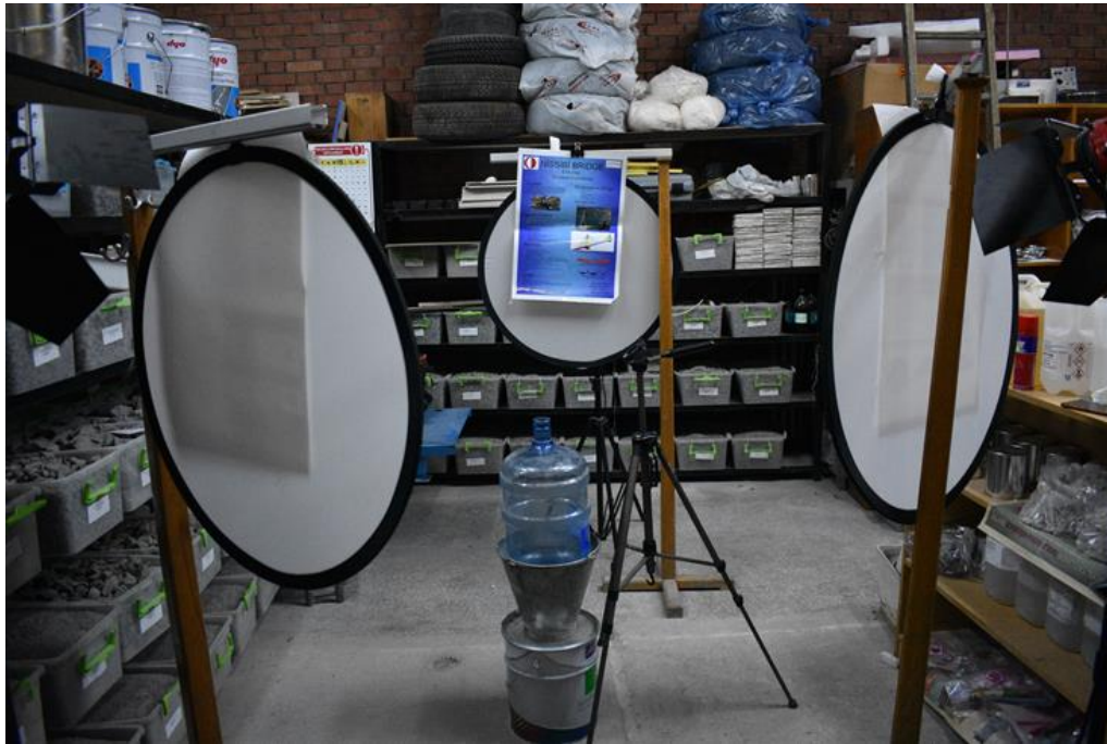
Figure 3.8 3D photogrammetry setup for shooting
