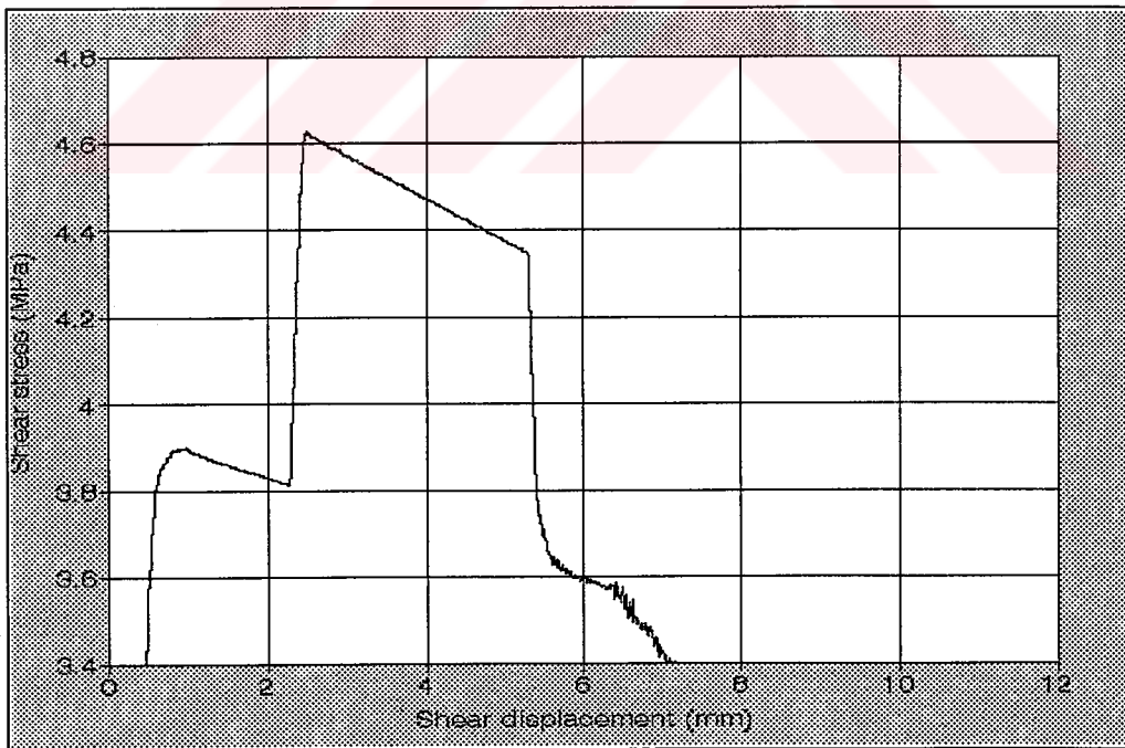
Figure 6.18 The shear stress vs. displacement of the stress step simulation (40% increment of normal stress)
