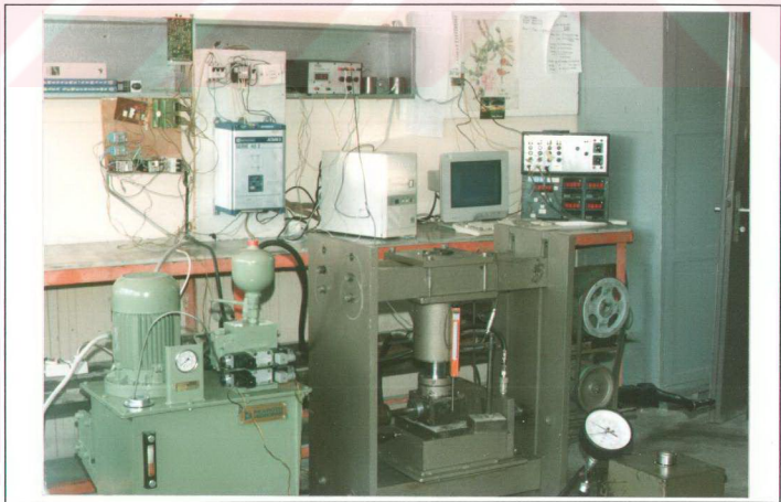
Figure 4.3 The general view of the computer controlled direct-shear apparatus
