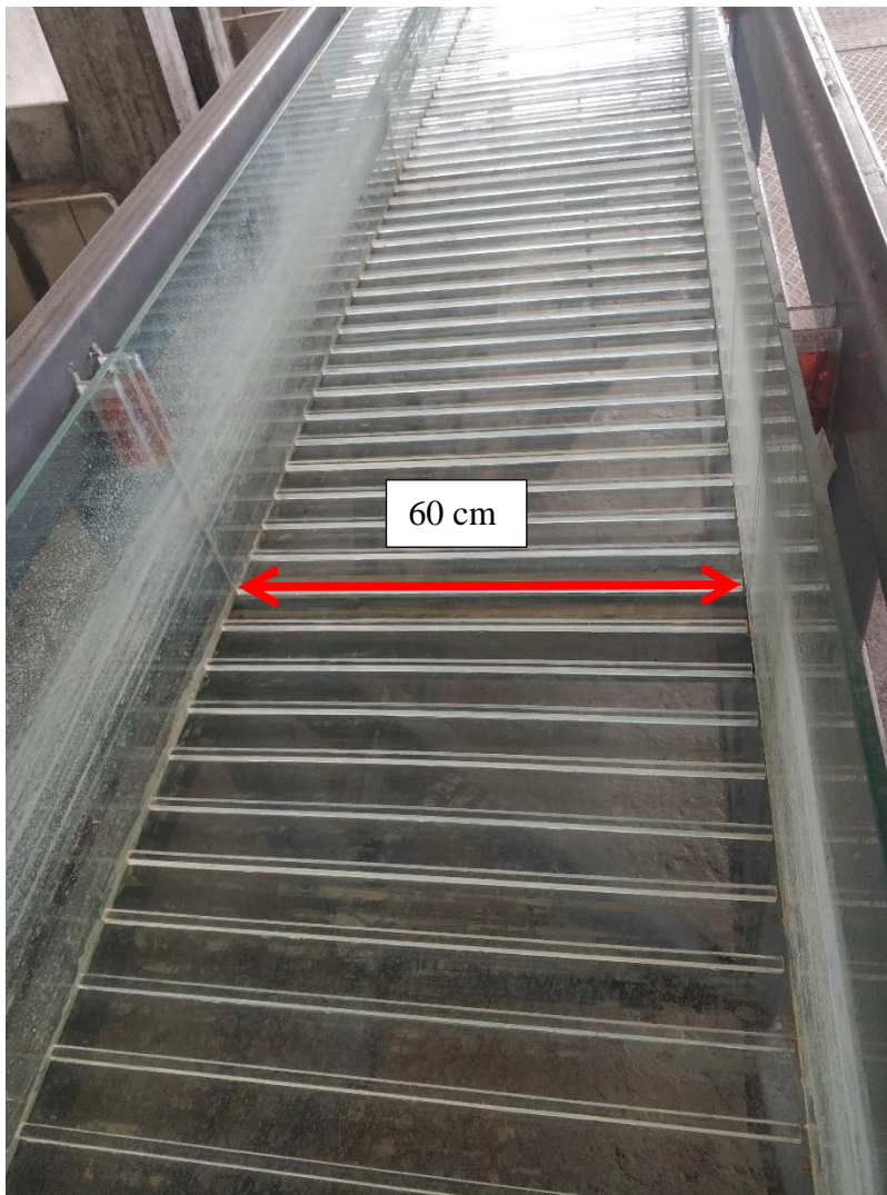
Figure 3.3 Square Bars Placed on the Channel Bed
