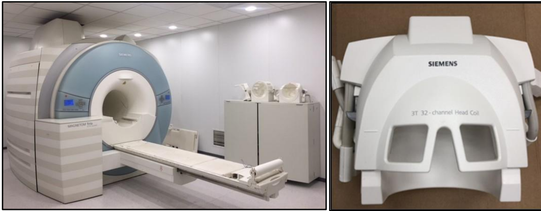
(A) (B) Figure 3.1: A) The fMRI scanning room at UMRAM B) The 32 channel head coil
