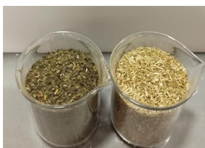
Figure 1. 6 The image of the green tea leaves (left side) and green tea waste fibers
