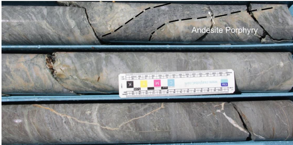
Figure 4-6. Schist unit with strong foliation intersected by quartz-feldspar porphyry in the study area (drill hole EU-046, 153.60 m.).
