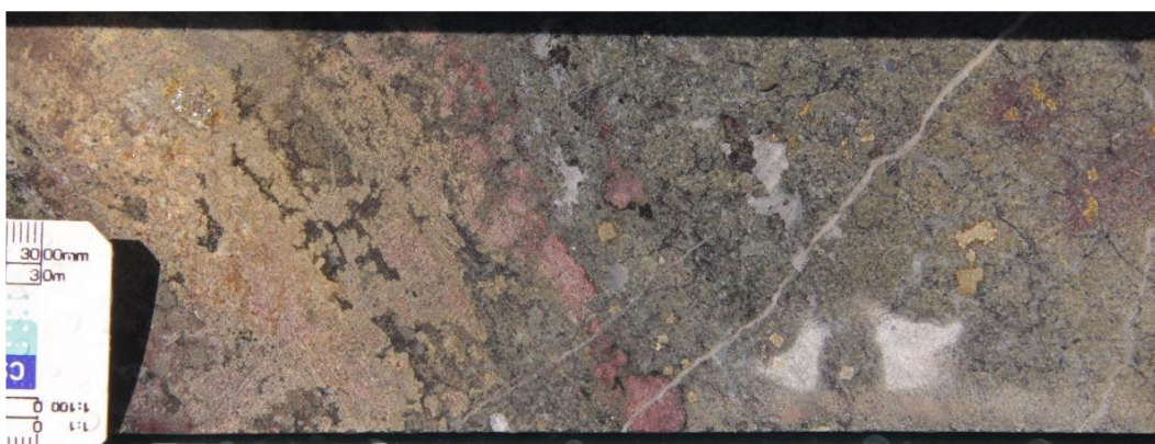
Figure 5-2. Yellowish brown colored garnet with greenish colored pyroxene skarn in the study area (drill hole EU051, 83.00 m)
