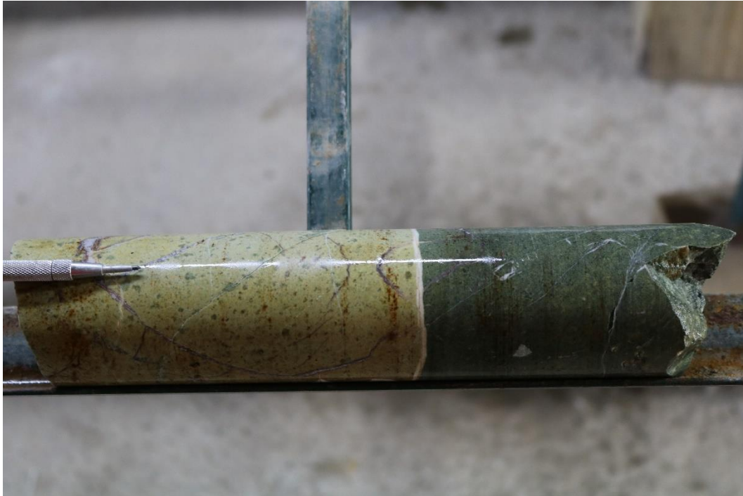
Figure 4-19. Drill core interval of andesite porphyry (left) cross-cut by a basaltic dike (drill hole EU-071, 50.70 m). Andesite porphyry shows intense carbonate-chlorite-sericite alteration, whereas the basaltic dike experienced intense chloritization as indicated by its distinct green color.
