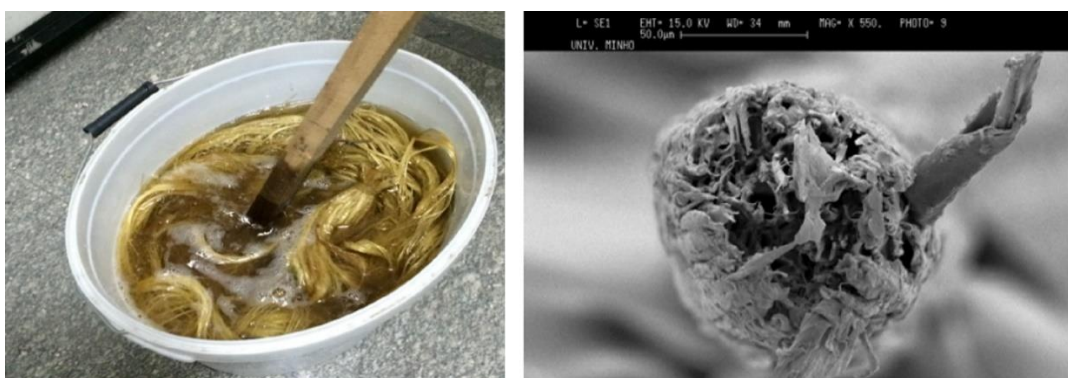
Figure 2.7 Banana fiber immersed into Sodium Hydroxide solution (left) (Mostafa & Uddin, 2015), SEM showing the cross-section of banana fiber (Mukhopadhyay et al., 2008)
