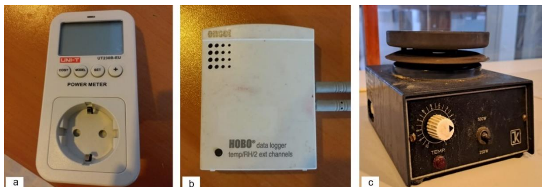
Figure 3.8 Materials used for experimental setup; a: power meter, b: HOBO data logger with temperature- relative humidity external channels and c: 500 W and 250 W Van der Heyden laboratory stove.
