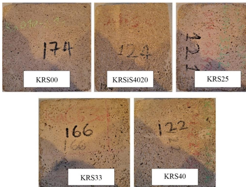
Figure 3.5 Samples stabilized with river sand, siliceous sand and straw; sample no. 174 of mix KRS00 reference sample (upper left), no. 124 of KRSiS4020 with 40% siliceous sand and 20% straw (middle), 121 of KRS25 with 25% straw, no. 166 of KRS33 with 33% straw (lower left) and no. 122 of KRS40 with 40% straw by volume (lower right)
