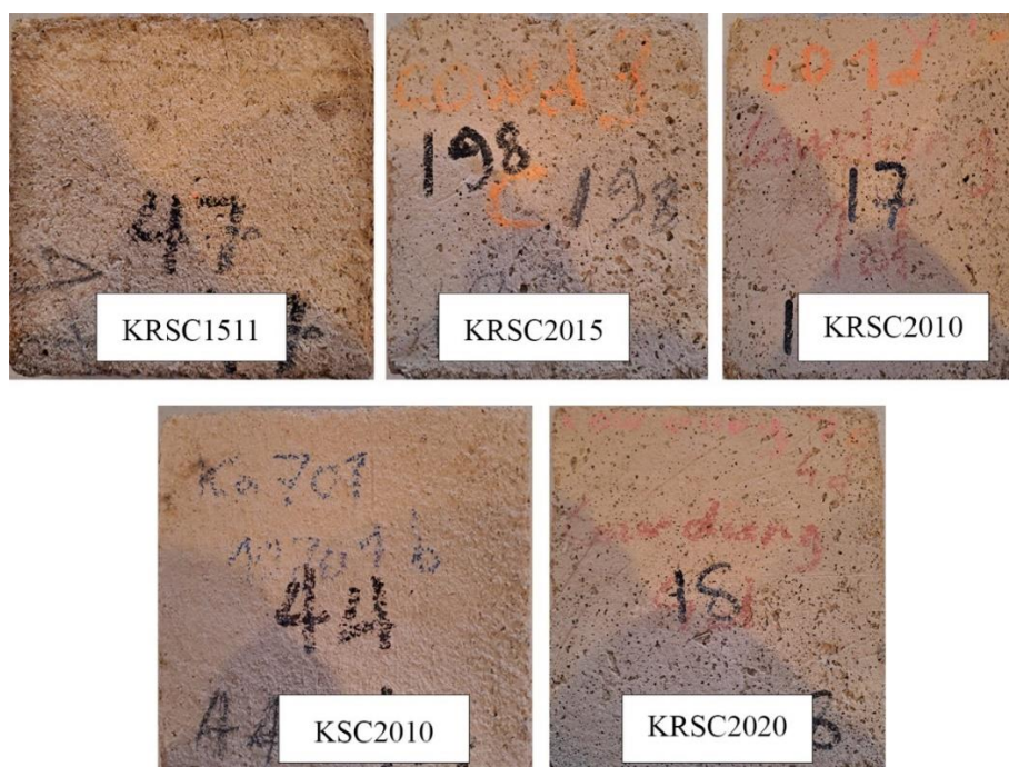
Figure 3.6 Samples stabilized with cow dung; sample no. 47 of mix KRSC1511 with 15% straw and 11% cow dung (upper left), sample no. 198 of mix KRSC2015 with 20% straw and 15% cow dung (middle), sample no. 17 of mix KRSC2010 with 20% straw and 10% cow dung (upper right), sample no. 44 of mix KSC2010 with 20% straw and 10% cow dung (lower left) and sample no. 18 of mix KRSC2020 with 20% straw and 20% cow dung by volume.
