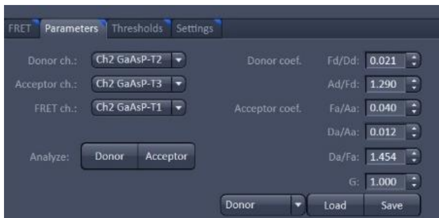
Figure 3.15 FRET parameters gathered from Zeiss LSM880 Laser Scanning Confocal Microscope Zeiss Zen Modul FRET plus Macro using the Xia et.al. method settings for donor bleed-through and direct acceptor excitation.
