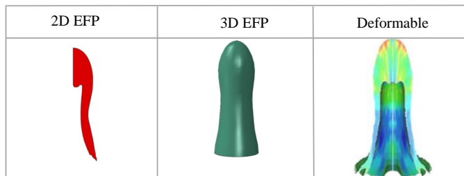
Figure 5.7: Formed 2D shape and 3D models of EFPs at the onset of impact with ABAQUS. Deformable EFP is from [88] with LS-DYNA.
