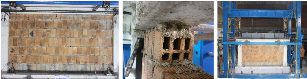
Figure 3.9. Construction of HCB infilled frame
