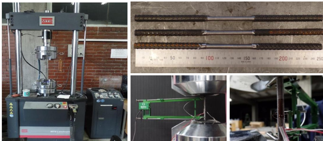
Figure 4.2. Uniaxial tensile testing of reinforcing bars
