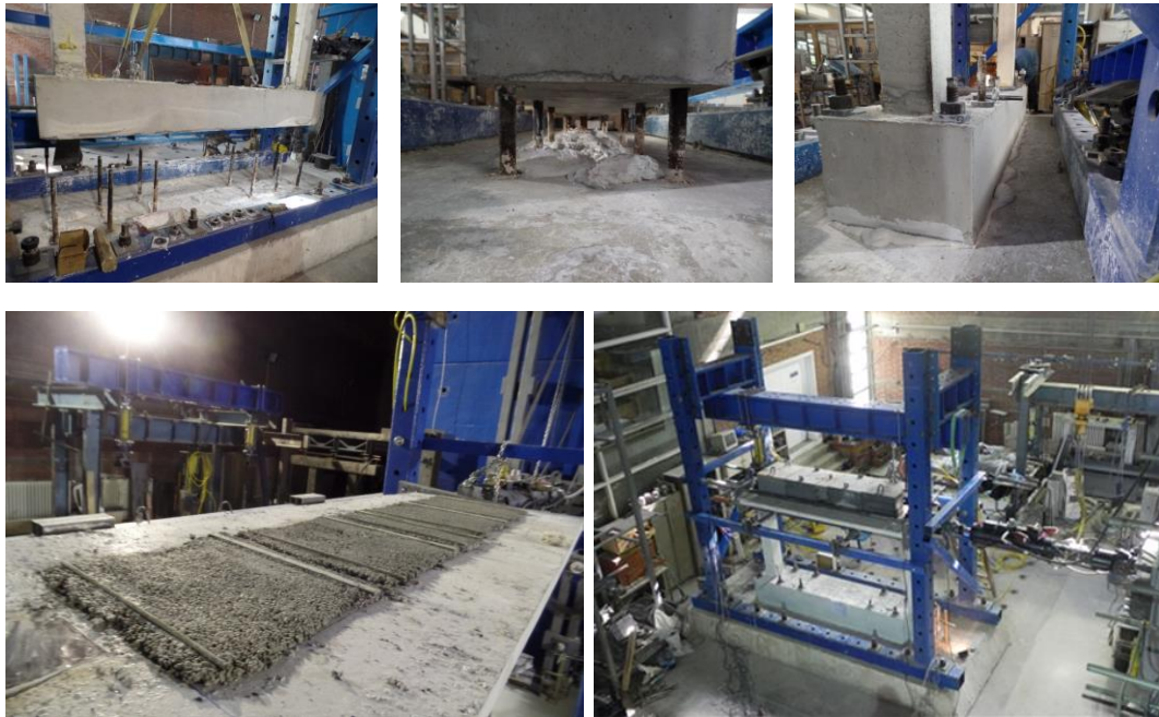
Figure 3.8. Placement of frame specimens on the transfer slab
