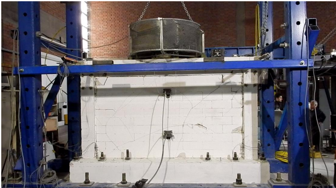
Figure 5.26. OOP testing of damaged AB frame with vibration generator
