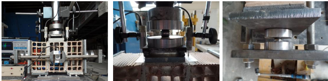
Figure 4.18. Sliding shear test of masonry prisms
