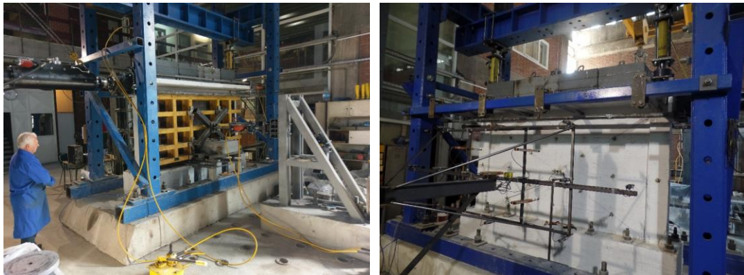
Figure 3.22. Out-of-plane testing setup
