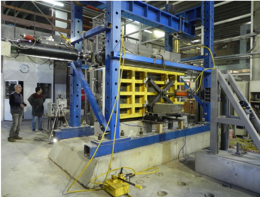
Figure 5.51. Test setup for combined IP and OOP loading of infilled frames
