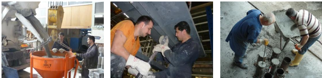
Figure 3.7. Concrete casting and sampling
