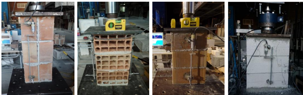
Figure 4.13. Uniaxial compression testing of masonry prisms
