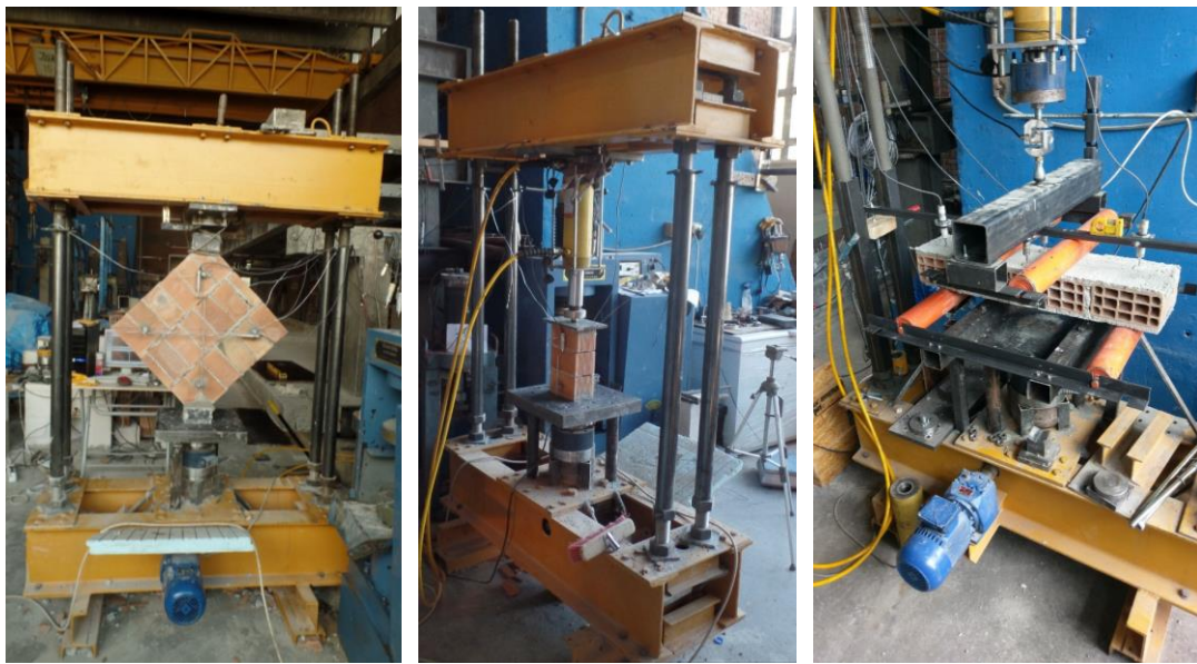
a) Diagonal tension b) Uniaxial compression c) 4-point bending
