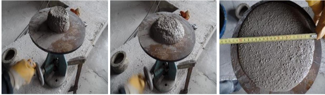
Figure 4.7. Flow tests conducted for mortar consistency
