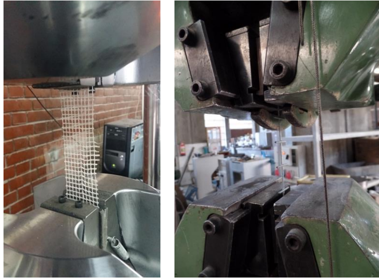
Figure 4.9. Testing of mesh reinforcement a) Fiber (Todorovic 2019), b) Steel
