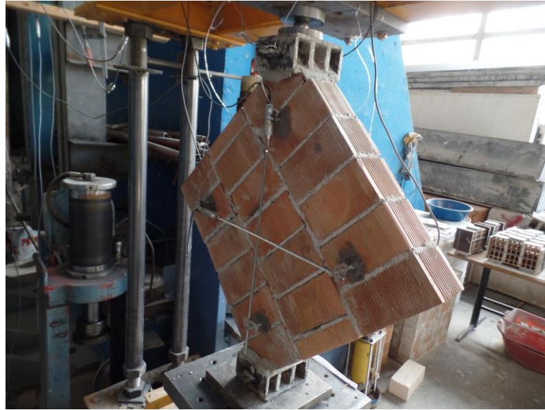
Figure 4.16. Diagonal compression test
