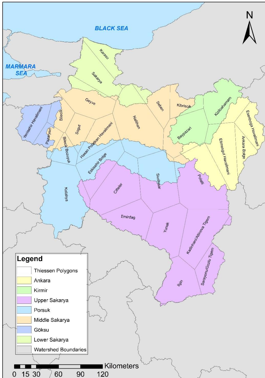
Figure 5-7. Thiessen polygons used to obtain climate data of catchment components in the WEAP model
