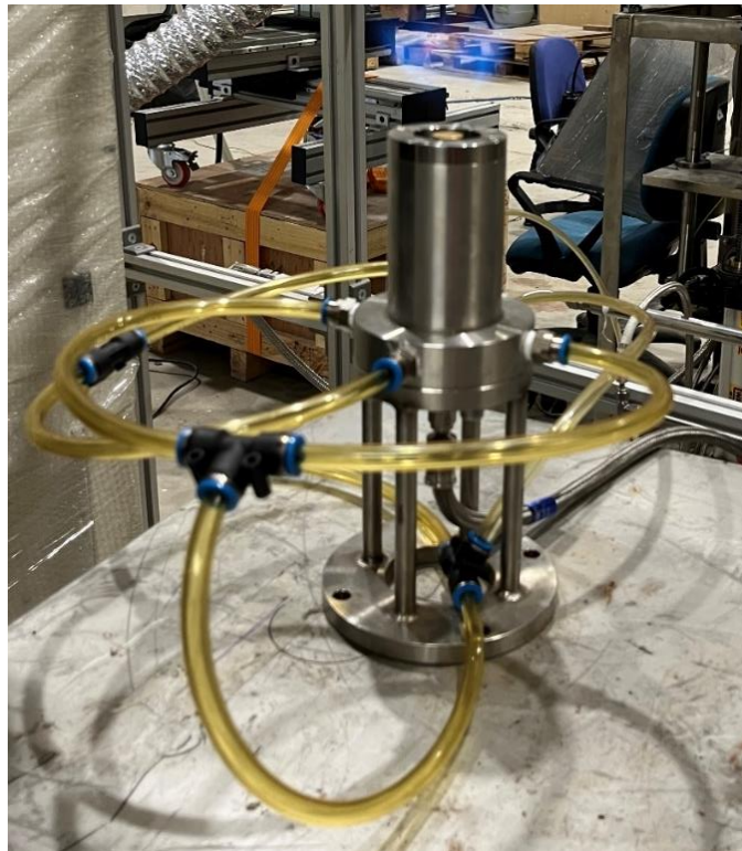
Figure 3.2. A photo of the experimental swirl burner
