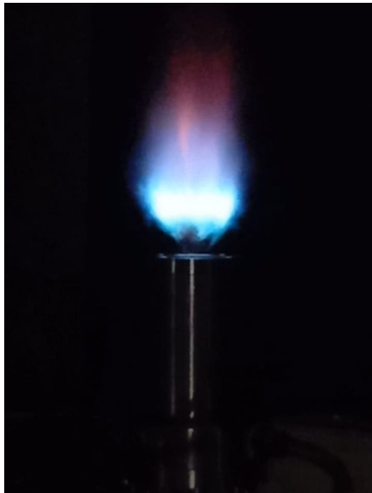
Figure 5.2. A picture of the lifted-off flame at 60 H 2 VOL%
