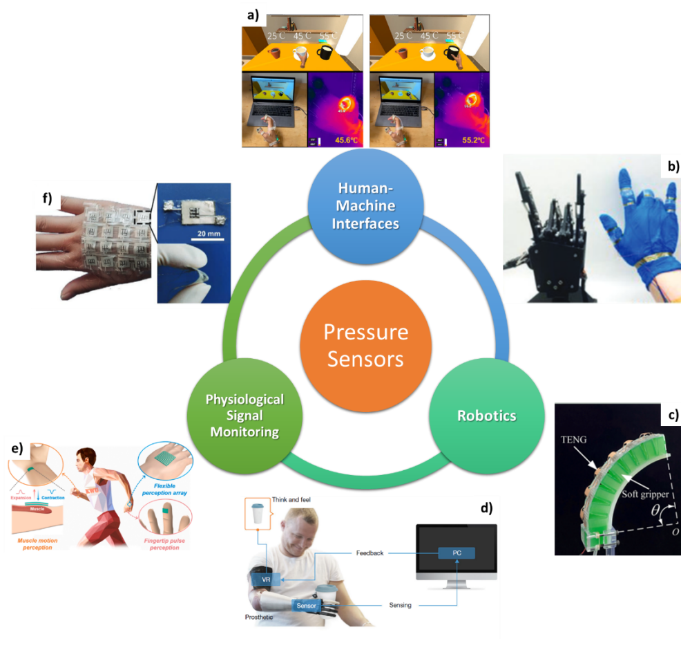
Figure 4.2 Main usage areas of pressure sensors and their related applications. a) Thermo-haptic feedback. [328] b) Controlling robotic arm using hand gestures. [329] c) Robotic gripper grasping system sensor. [330] d) Prosthetic arm with an epidermal VR [331] . e) Tactile sensor for physiological signal sensing. [332] f) Bimodal sensor array attached on hand [333] .
