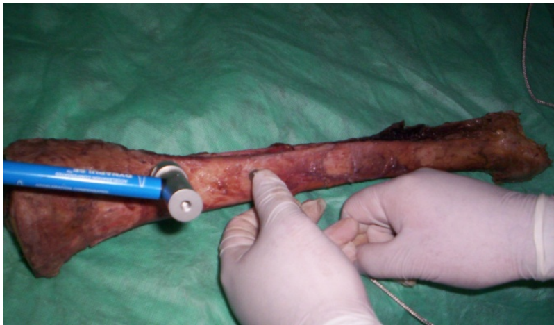
Figure 1. Measurement of FRFs on fresh-frozen tibial bone
