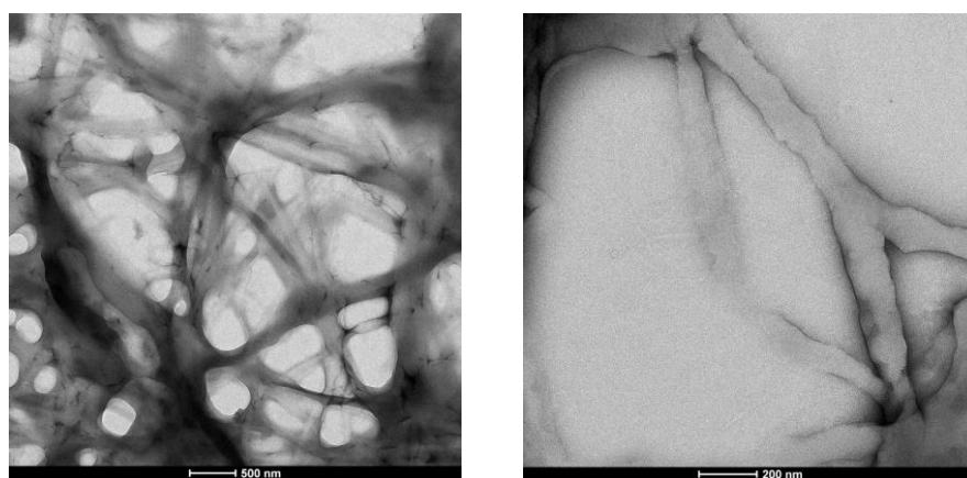
Figure 10: TEM images of 5 wt/v% L-Cys( St Bu)-OH based organogel in THF.
