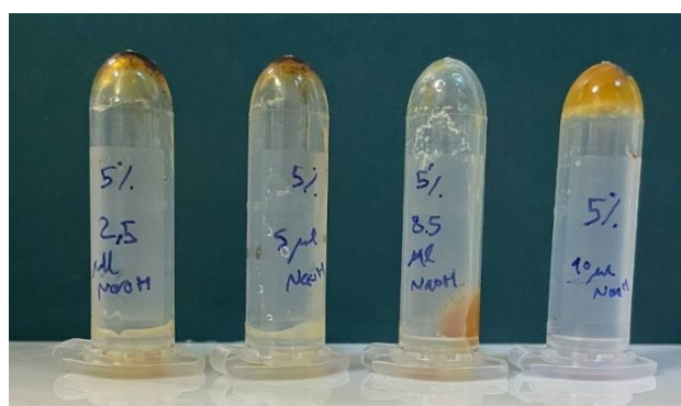
Figure 8: 2.5, 5, 8.5, and 10 \mu L of 10 M NaOH used for 5 wt/v% L-Cys( t -dodecyl-sulfanyl)-OH based gel formation in sunflower oil.
