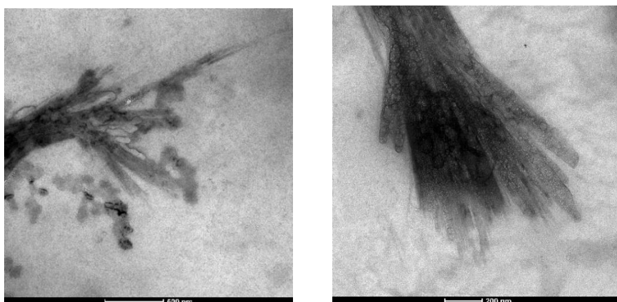
Figure 11: TEM images of 5 wt/v% L-Cys( t -dodecyl-sulfanyl)-OH based organogel in sunflower oil.
