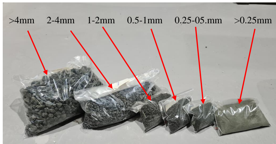
Figure 3.15. Clinker sieved and packed
