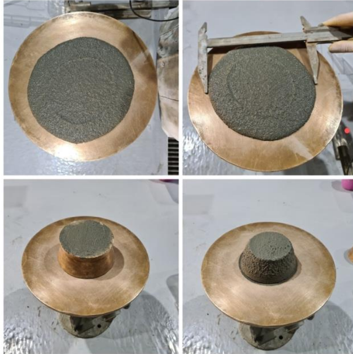
Figure 3.11. Cement mortar before (below) and after (above) spreading during the flow table test
