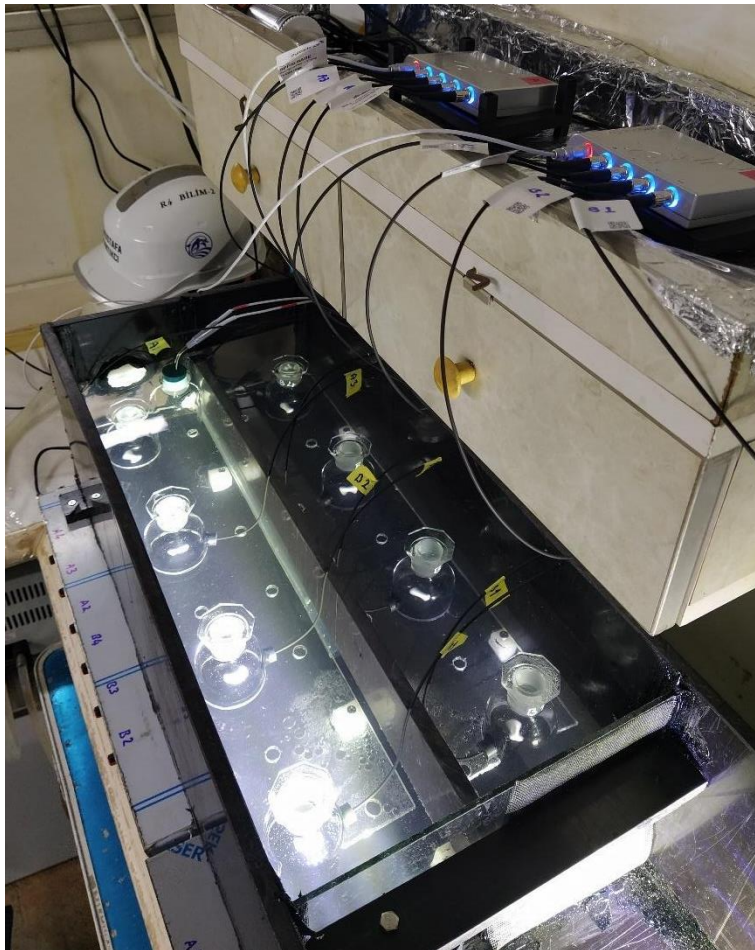
Figure 2.6 OPTODEs and temperature controlled linear light on and dark incubator system
