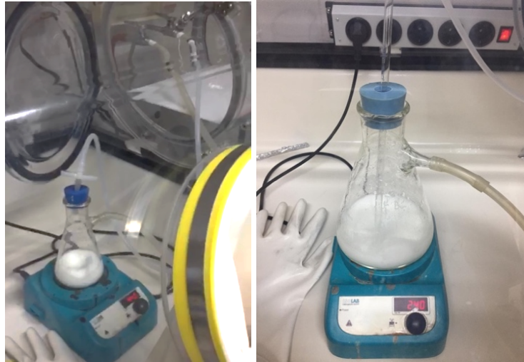
Figure 3.1 Preparation setup of crystalline cellulose solution
