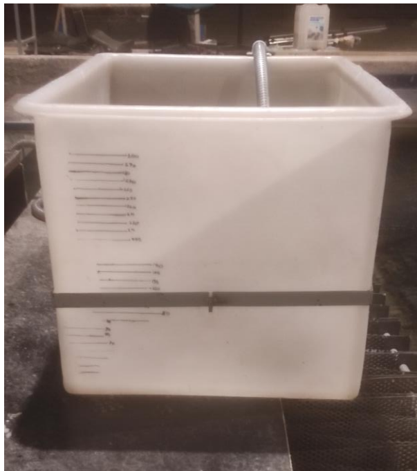
Figure 3.7 Overtopping collection tank
