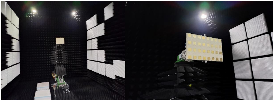
Figure 4.33. Radiation pattern measurements in the anechoic chamber
