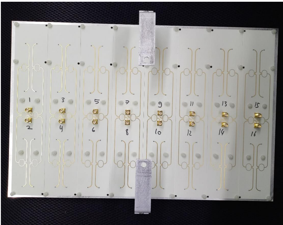
Figure 4.22. Bottom view of prototype antenna array
