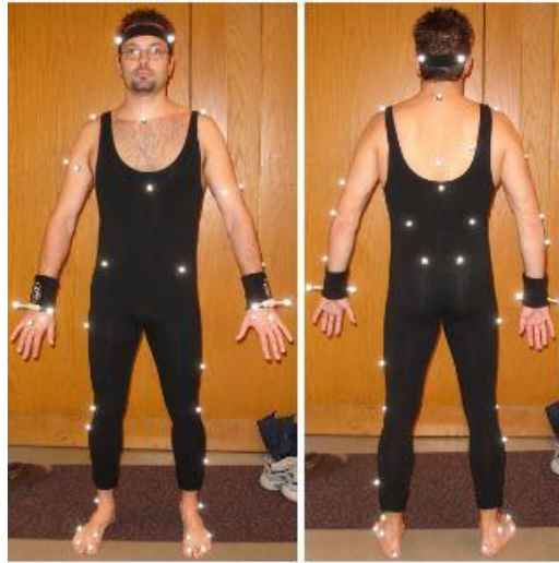
Figure 3.1. The Jumpsuit Used by CMU-GL, Having 41 Markers Taped on (Retrieved from mocap.cs.cmu.edu)
