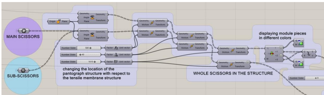
Figure 3.23. The Grasshopper Script of Connecting All Scissors to Create the Overall Pantograph Structure
