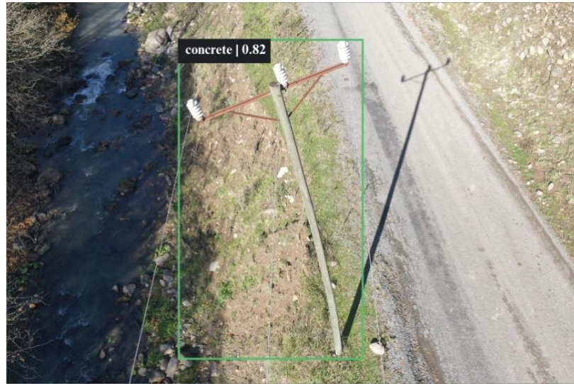
Figure 52. Incorrectly Classified Wooden Pole
