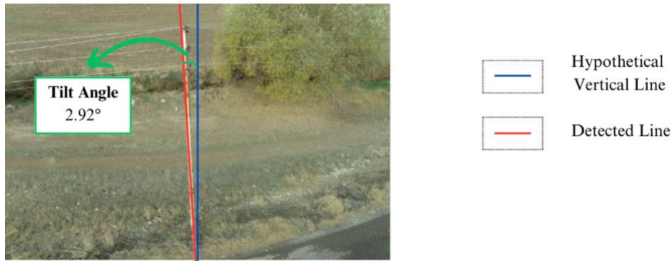
Figure 47. Example Measurement of Tilt Angle
