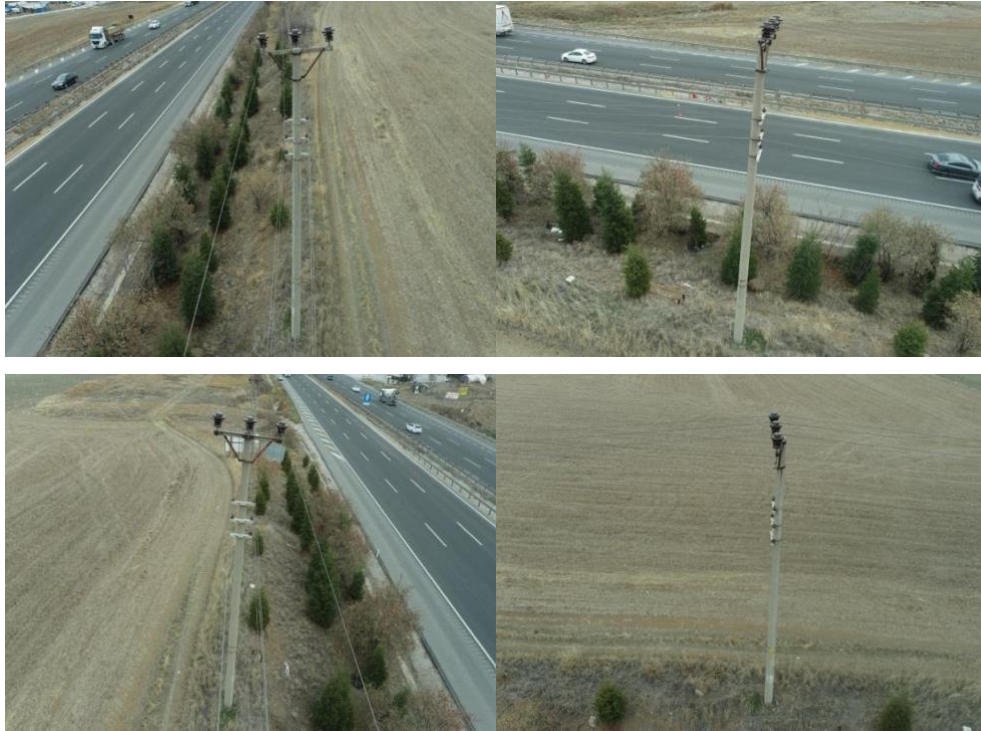
Figure 51. Images Collected for the Detection of Tilted Electricity Poles
