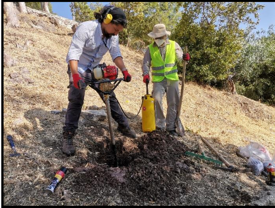
Figure 3.2 Soil sampling with a portable drilling machine.
