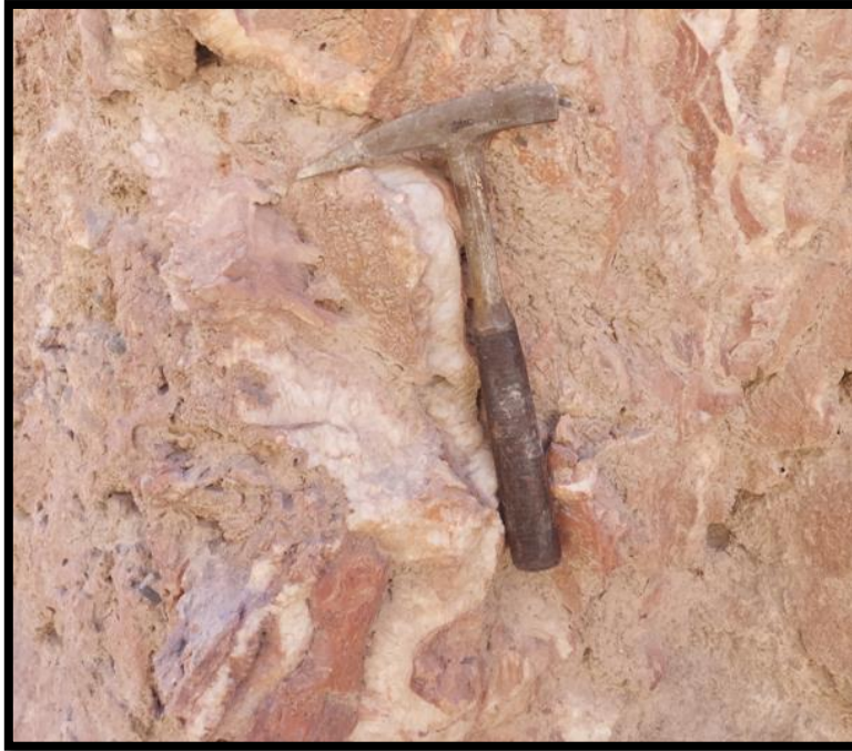
Figure 6.3 Recrystallized aragonite mineralization in limestone blocks from the quarry located in easter part of İzmir and Bornova (38.4629167, 27.3102511) with values of As=79.5, Cd=0.14, Co=2.18, Ni=8.06, Sb=2.08, Zn=29.5 ppm.
