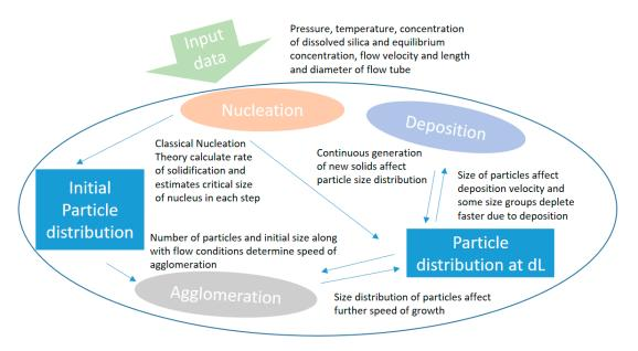
Figure 4. Schematic illustration of simulation process.
