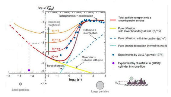
**Figure 3.** Particle deposition velocity at varying relaxation times as presented in reference [50] including data presented in [51,53].
