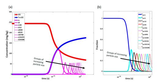
**Figure 7.** (a) Actual concentration and (b) fraction of concentration in each group as function of time. On the left plot (a), the blue line shows increase in total solids in the solution. The pink lines represent concentrations in groups of increasing size. As agglomeration evolves, the concentration in the smaller-sized groups decreases in favor of the larger-sized groups. On the right side (b), the increasing group size is given in different colors. The trend is, however, the same.
