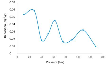
**Figure 12.** Expected deposition profile in a cascade of pressure drops calculated using the model presented in this paper with process conditions and silica content similar to the experimental conditions.
