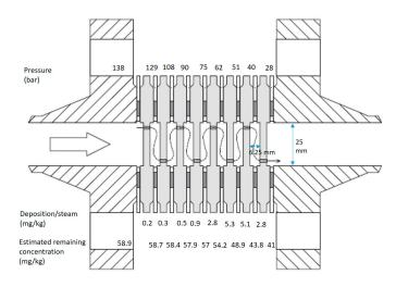
Figure 11. IDDP1 scaling experiment with cascading orifices.
