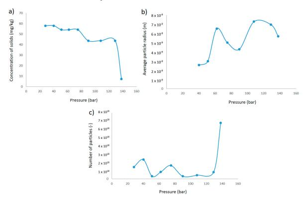
**Figure 13.** (a) Concentration of solids in the solution in each pressure reduction section just before entering the next orifice. (b) Average radius at the end of each pressure reduction section and (c) Average number of particles at the end of each section.
