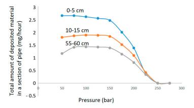
**Figure 9.** Change in deposition rate as a function of pressure reduction/supersaturation in specific 5 cm sections of pipe starting first initially downstream the pressure drop (blue), then 10 cm downstream of the pressure drop (orange) and finally 55 cm downstream of the pressure drop (grey).
