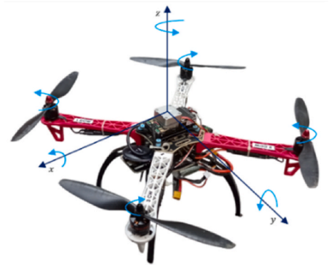
Fig. 10. Photograph of the fully assembled quadcopter [33].
