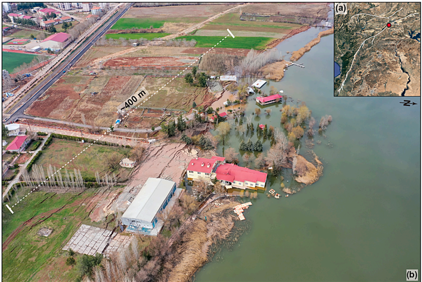
Fig. 13. Drone image showing an area affected by lateral spreading (lat: 37.79°, lon: 37.65°) near Golbasi, Adiyaman. The red point in panel (a) shows the landslide location. Panel (b) shows the area from the top with a bar scale. (For interpretation of the references to colour in this figure legend, the reader is referred to the web version of this article.)
