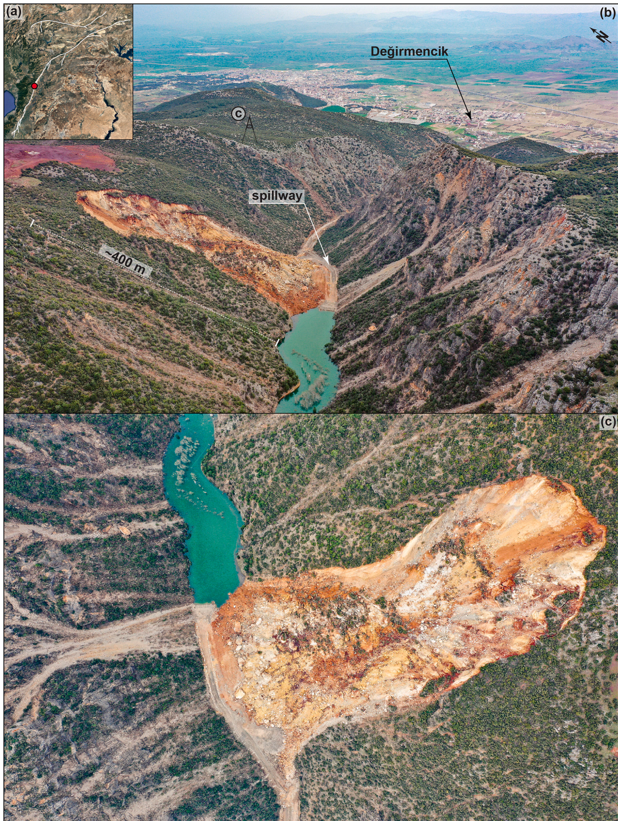
Fig. 18. Aerial photos showing an example of a landslide dam (lat: 37.00°, lon: 36.59°) near Islahiye, Gaziantep. The red point in panel (a) shows the landslide location. Panel (b) and (c) show landslide body from different angles. The viewing angle of panel (c) was indicated in panel (b). (For interpretation of the references to colour in this figure legend, the reader is referred to the web version of this article.)
