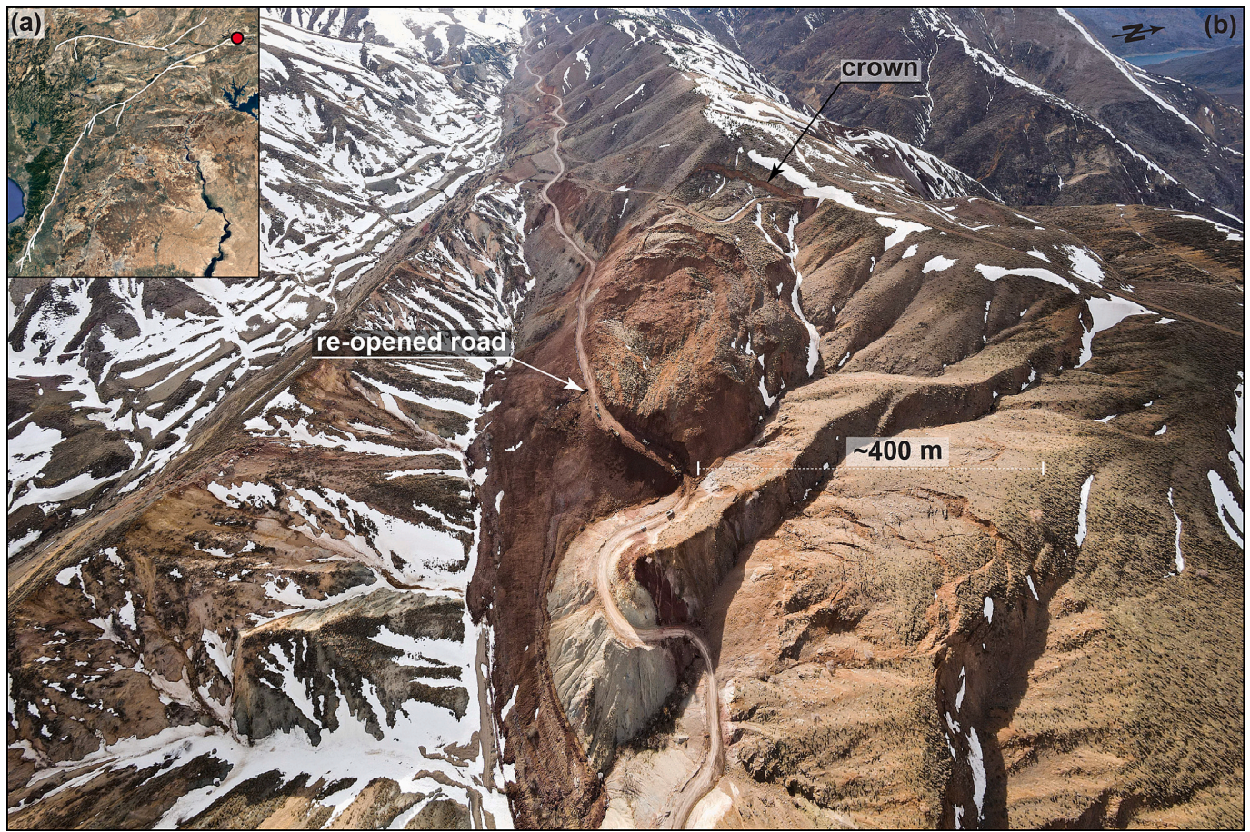
Fig. 17. View of the main road connecting the mountainous hamlets and district blocked by coseismic landslides (lat: 38.05°, lon: 38.36°) near Adiyaman. The red point in panel (a) shows the landslide location. Panel (b) shows the road, failed landslide and crown cracks. (For interpretation of the references to colour in this figure legend, the reader is referred to the web version of this article.)
