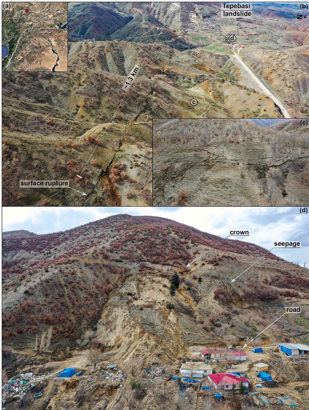
Fig. 14. Drone images showing a coseismic landslide occurred along the surface rupture (lat: 38.06°, lon: 36.99°) near Ekinözü, Kahramanmaraş. The red point in panel (a) shows the landslide location. Panels (b-c) and (d) show surface rupture and zoom-in view of landslide location, respectively. The viewing angles of panels (c) and (d) were indicated in panel (b). (For interpretation of the references to colour in this figure legend, the reader is referred to the web version of this article.)
