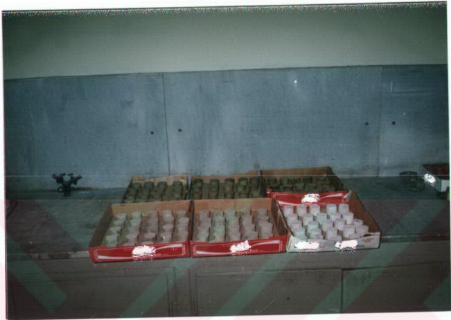
Figure 9 : Dried Bricks Containing Tailing Clay
