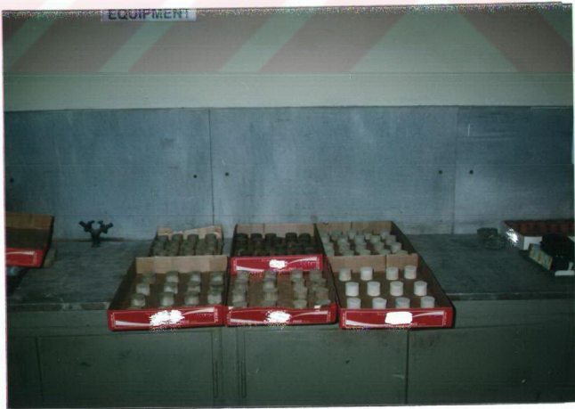
Figure 10 : Dried Bricks Containing Calcined Tailing Clay
