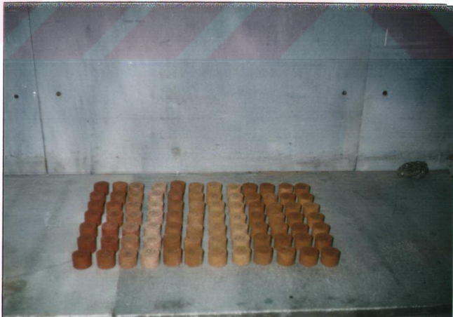
Figure 12 : Fired Bricks Containing Calcined Tailing Clay
