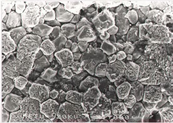
Figure 5.2. SEM micrograph of the ceramic sample with 0.25 atomic percent \text{La}^{+3} and 0.04 atomic percent \text{Mn}^{+2} additions.
