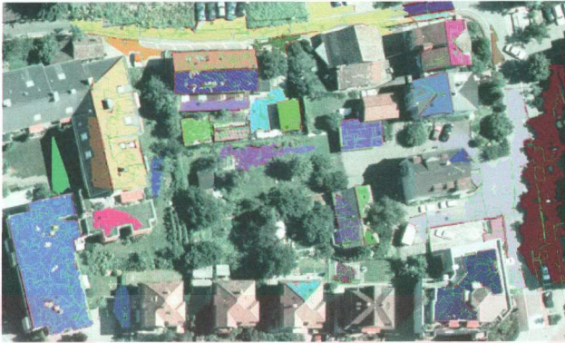
Figure 4.15: Reconstructed surfaces re-projected on Zürich image. Each surface is shown in a different color.
