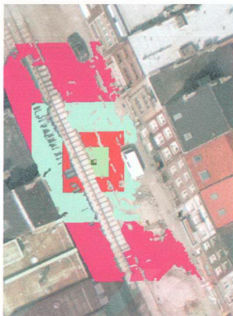
Figure 4.8: Four stages of surface growing coded in different colors. The evolution of the error function is inspected during the surface growing process.
