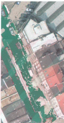
Figure 4.11: The largest surface patch projected on one of the Brussels images. This surface is used for analyzing the error distributions and photometric distortion.
