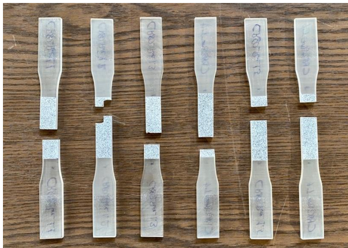
Figure 2.18. Fractured CR80 resin system dogbone specimens after tensile testing.
