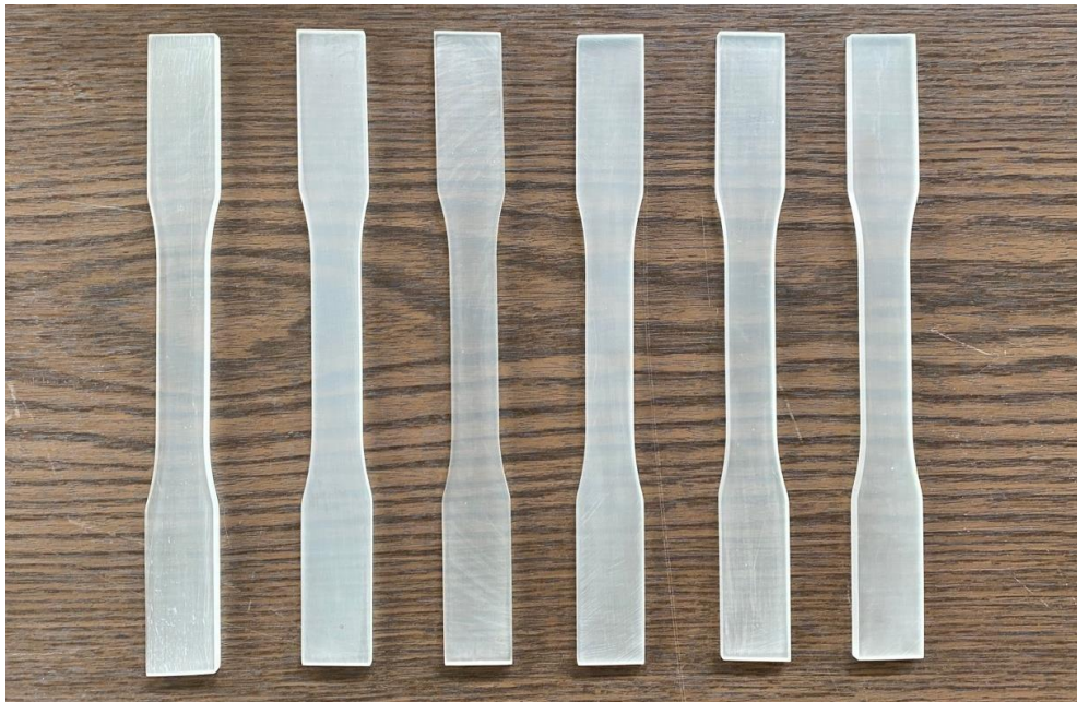
Figure 2.17. The dogbone tension specimens after the manufacturing process.
