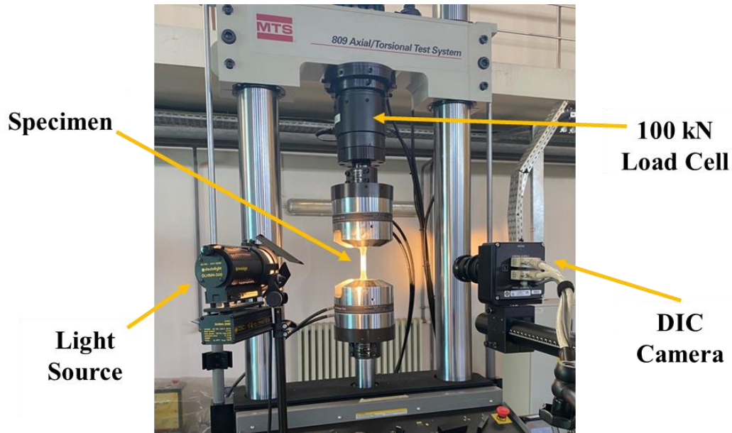
Figure 2.3. Test setup for the tension tests.
