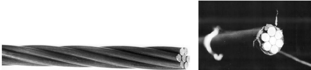
Figure 2.13 Seven Wire Strand (Gimsing & Georgakis, 2012)
