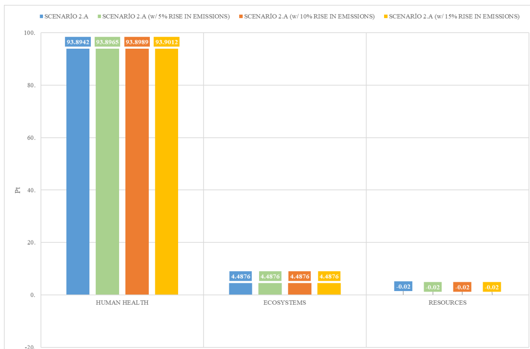
Figure 4.15 Comparative end-point single- score results for variation in emission levels to soil.
